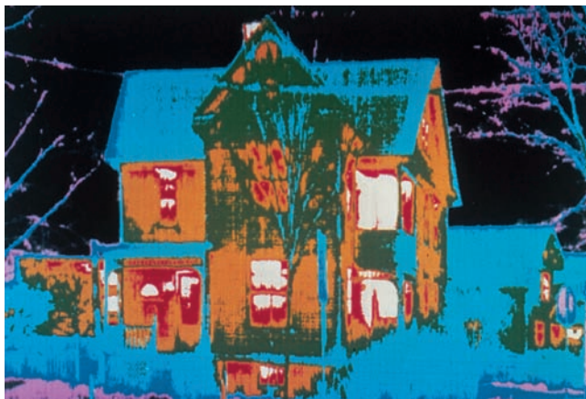
figure 1.8 An infrared photograph showing patterns of heat loss from a house is an application of thermodynamics.
